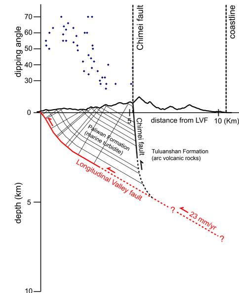
Figure 10. Reconstruction of the subsurface geometry of the Longitudinal Valley fault near Hsiukulan canyon, from bedrock dip angles. The azimuth of the section is approximately N80W. This model indicates that the slip rate on the fault is about 23 mm/yr and that all of the deformation is accommodated by the slip along the fault plane, with no internal deformation of the beds.
