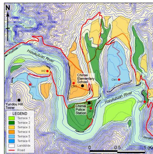
Figure 8. Detailed map of river terraces in Chimei area, showing the distribution of terraces and pit locations. Thin dashed lines are the boundary of terrace surfaces, and bold lines show the strath of terraces, wherever visible in the field.
