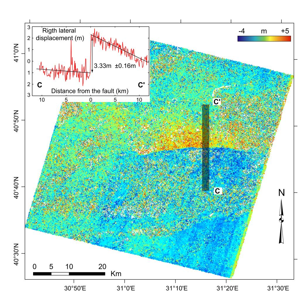
East-West component (eastward positive) of the ground displacement measured between a SPOT 1 image acquired on the 10/03/1999, and a SPOT 4 image acquired on the 07/12/2000. These images bracket only the Duzce event, so that only the coseisimic displacement induced by the Duzce earthquake is analysed. This correlation image clearly indicates where the Duzce rupture starts. The profiles BB' and CC' also highlight the consistency of the measurements
