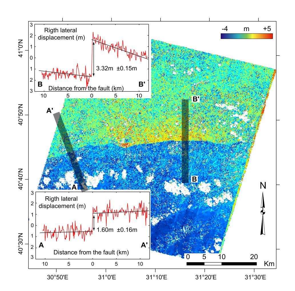
East-West component (eastward positive) of the ground displacement measured between a SPOT 1 image acquired on the 06/26/1999, and a SPOT 4 image acquired on the 07/12/2000. The Izmit earthquake occured on the 08/17/1999, and the Duzce earthquake on the 11/15/1999. This image then reprensents the cumulative coseismic displacement due to both events. The continuity of the ruptures is here evident, and the ground rupture can be traced all the way east where it has been missed during field surveys.
