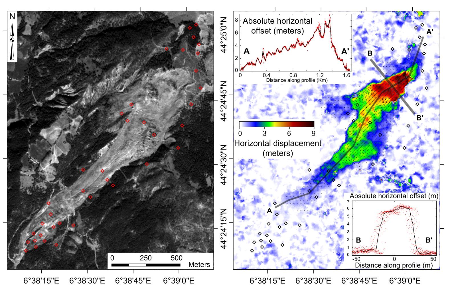
(left) Orthorectified SPOT image of the La Valette landslide. The red diamonds show the geodetic benchmarks for field survey.
