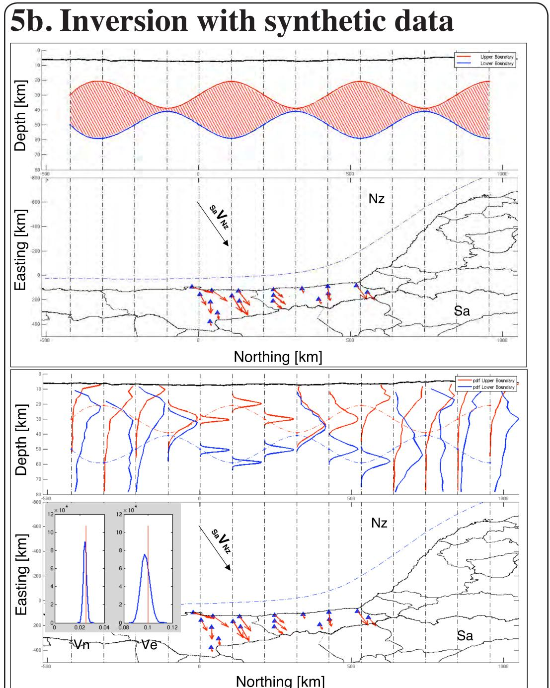
We perform a synthetic test to our inversion method using the model in the upper panel of figure 5b. The results of the inversion are shown in the bottom panel of figure 5b. Note that the target model is being recovered by the inversion process and the precision is highly dependent on the spatial distribution of the GPS stations.
