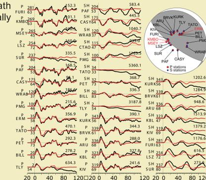
**Figure 7 | Mw7.9 joint inversion model fits to the teleseismic data.** Observed (black) and synthetic (red) teleseismic P and SH waveforms. Station name, azimuth, and distance are indicated on the left of each trace. The maximum displacement is shown at the top right of each trace in microns.
