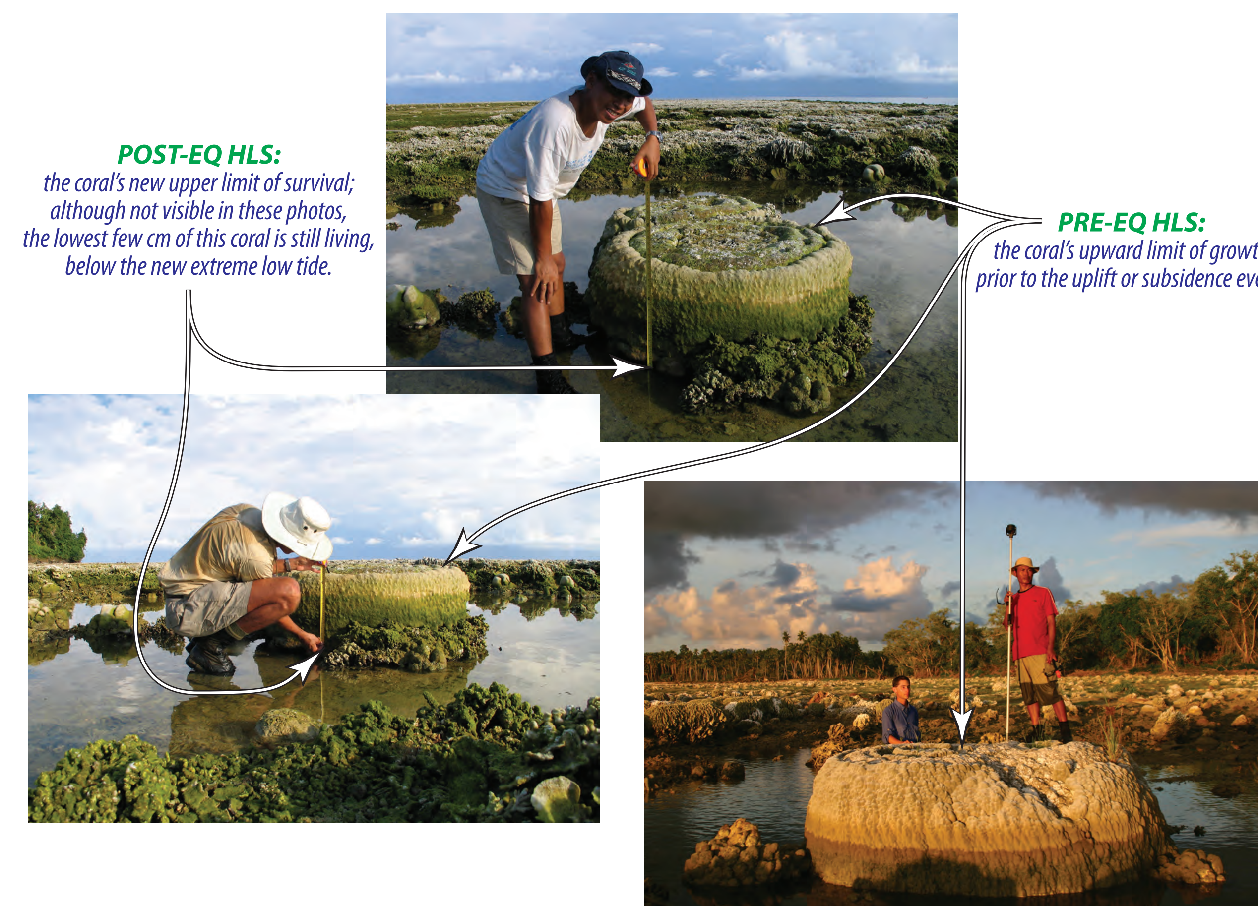
Scenarios for measuring vertical deformation using coral microatolls. (A) Uplift recorded as the difference between pre- and post-earthquake highest level of survival (HLS). (B) Uplift as separation between pre-earthquake HLS (pre-EQ HLS) and the post-earthquake annual extreme low tide (post-EQ ALT), determined by (a) surveying the water level at any given time; (b) noting the exact time of measurement; and (c) using a computational tide model and sea-level anomalies to tie the water level measurement to the lowest water level of the year.
