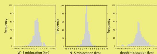
**B)** Shows the difference in event locations between locations in the original and rotated 2D velocity model.
