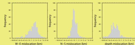
**A)** Shows the difference in event locations between locations in a 1D and 2D velocity model.
