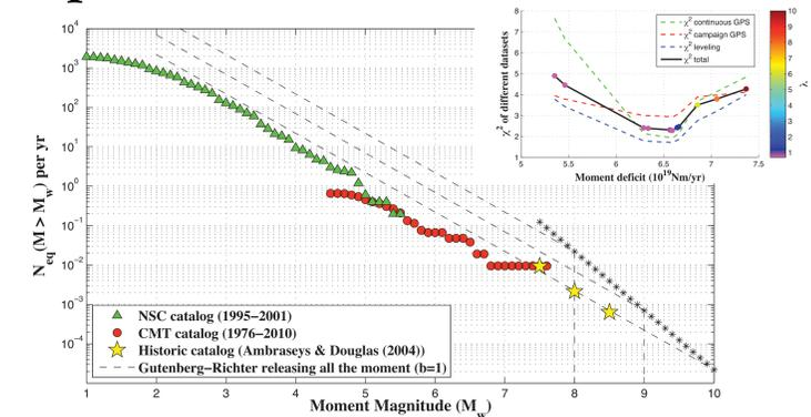
**Inset:** Impact of the weights applied to the Laplacian. The plots show the value of the reduced  $\chi^2$  of the fit as well as the moment deficit accumulation rate for each inversion. The best fitting model has a moment deficit rate of  $6.6 \pm 0.4 \times 10^{19} \text{ Nm/yr}$ .
