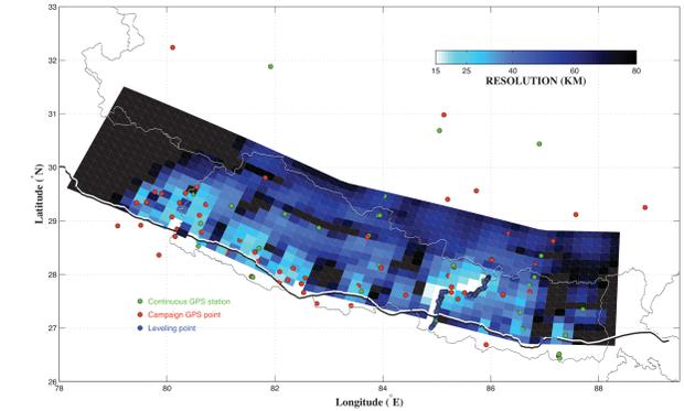
Resolution on each of the patches of the fault, given in km. This resolution size measures the distance over which the slip on a patch is affected by the slip on its neighboring patches. Locations of the data points used to compute the resolution are indicated in the figure and legend.
