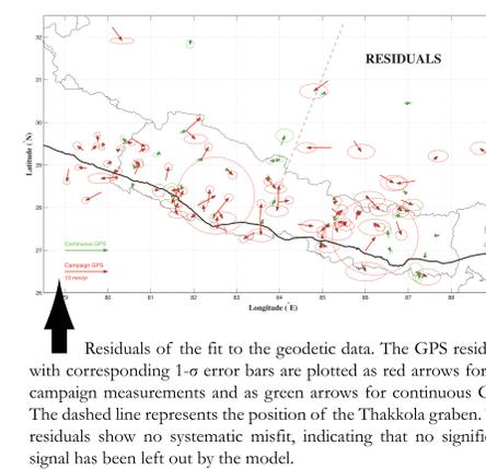
Residuals of the fit to the geodetic data. The GPS residuals with corresponding 1- $\sigma$  error bars are plotted as red arrows for the campaign measurements and as green arrows for continuous GPS. The dashed line represents the position of the Thakkola graben. The residuals show no systematic misfit, indicating that no significant signal has been left out by the model.
