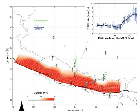
Fit to the continuous GPS vertical velocities (map) and to the spirit leveling data (inset). White dots show location of the leveling line. The inset shows the fit to leveling data.
