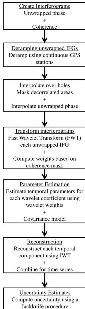
Figure 1. Detailed flowchart of the various processing stages in our MInTS analysis of the InSAR data sets [1].
