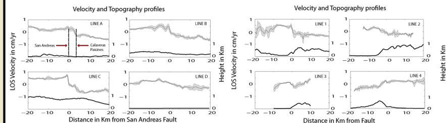
Figure 3. LOS velocity profiles (shaded) and topography profiles (solid) plotted along the dotted lines across the San Andreas Fault as shown in Figure 2. A region of 6 km was averaged along the profile lines.
