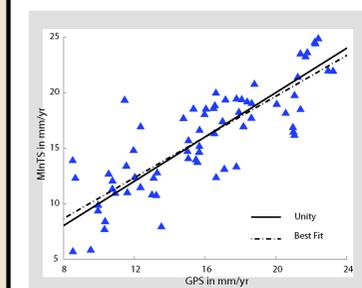
Figure 5. Comparison of MInTS LOS velocity estimates with GPS velocities projected into the satellite LOS for 69 PBO stations. The vertical components of the GPS were ignored and only the horizontal components were used for the comparison. Best fit line has a slope of 0.98 and rms value of 2mm.
