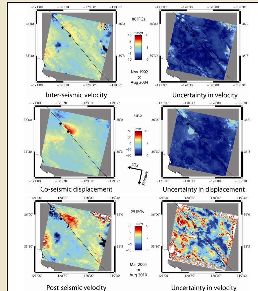
Figure 6. Estimated MInTS parameters and associated uncertainties for the C-band stack around Parkfield, CA. The epicenters of the 1966 and 2004 earthquakes are also shown. The number of interferograms and time-span of each of the stacks is also shown. The co-seismic displacements shown includes the rapid deformation (1 month time-scale) following the 2004 earthquake.
