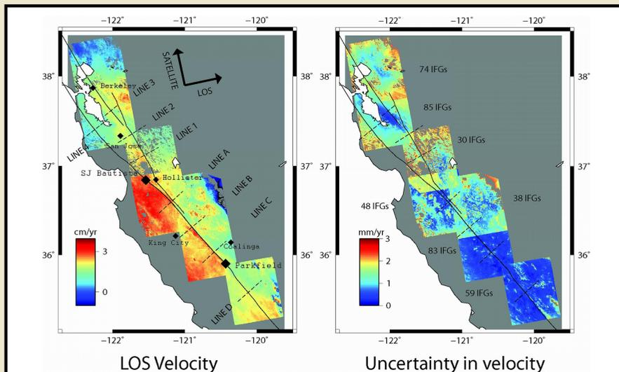
Figure 2. LOS velocity (Left) and the associated uncertainty (Right) mosaics of 7 different ALOS PALSAR frames covering Central California. The USGS traces for the San Andreas, Calaveras and Hayward Faults are also shown. 8 dotted line segments represent the location of the velocity profile lines shown in Figures 3 and 4. Number of interferograms used to generate the velocity map is also indicated in the uncertainty plot (Right).
