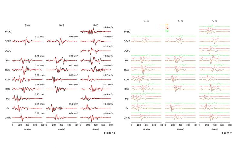
Figure 10. Regional waveform fits for the joint inversion model. In which data is shown as black and synthetic as red. All waveforms are filtered to 50s and longer using the same filter as in Fig.2. Station names are indicated at the beginning, the number at the end of each pair is the maximum amplitude of data. The empty spaces are clipped components.
