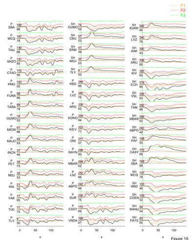
Figure 15. Separation of teleseismic waveform fits. Separation of teleseismic synthetics (gray) into the contribution of fault segment F1 (brown), F2 (red) and F3 (green). The empty spaces are clipped components.
