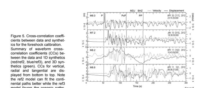
Figure 5. Cross-correlation coefficients between data and synthetics for the foreshock calibration. Summary of waveform cross-correlation coefficients (CCs) between the data and 1D synthetics (red/ref2, blue/ref3), and 3D synthetics (green). CCs for vertical, radial and tangential are displayed from bottom to top. Note the ref2 model can fit the continental paths better while the ref3 model favors the oceanic paths, separated by the dashed line.
