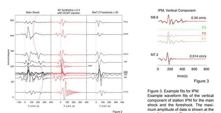
Figure 3. Example fits for IPM. Vertical component of station IPM for the main shock and the foreshock. The synthetic (gray) for the main shock is decomposed into the contribution from F1 (brown), F2 (red) and F3 (green). Note the synthetic for the foreshock is generated by the GCMT solution. All the synthetics are filtered to 50s and longer using the same filter as in Fig.2.
