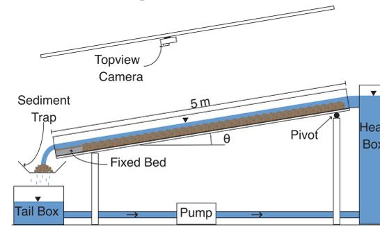
To address this gap in threshold of motion data we conducted laboratory flume experiments at 15 different slopes ranging from 3° to 33°. We used 1.5-cm siliclastic gravel sieved to a planar initial bed topography. Flow discharge was slowly increased until transport conditions were achieved. Flow velocity, discharge, and depth, as well as sediment flux were measured at each discharge in order to calculate the critical conditions.
