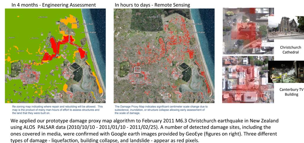
We applied our prototype damage proxy map algorithm to February 2011 M6.3 Christchurch earthquake in New Zealand using ALOS PALSAR data (2010/10/10 - 2011/01/10 - 2011/02/25). A number of detected damage sites, including the ones covered in media, were confirmed with Google earth images provided by GeoEye (figures on right). Three different types of damage - liquefaction, building collapse, and landslide - appear as red pixels.
