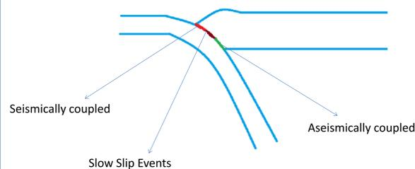
Figure 1: Subduction Zone with seismogenic interface
