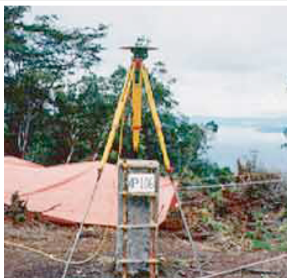
The image of an old primary triangulation pillar from the 1880s being surveyed by a GPS instrument in 1989. Monuments such as these, surveyed between 1989-2001, were resurveyed after the 2004 Sumatra-Andaman earthquake to determine coseismic displacements.
