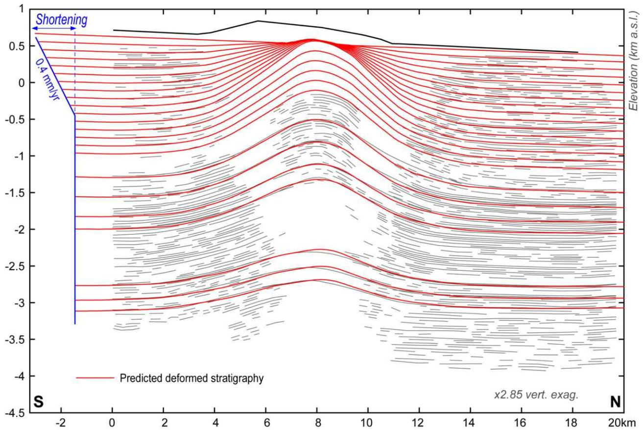
Figure 16: Predicted structure of Anjihai fold assuming a constant ratio of shortening versus sedimentation rates. This model predicts only negligible topographic relief, at odds with observed morphology.
