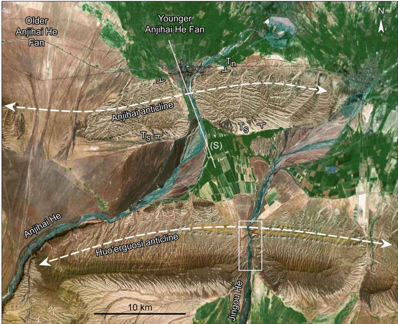
Figure 10: Map of Anjihai. Solid white line (S) marks location of seismic profile [Dengfa et al., 2005]. White “T” marks indicate dips of abrasion terraces T<sub>n</sub> and T<sub>s</sub>. White box shows the location of magnetostratigraphic section of Charreau [2005] across Huo’erguosi anticline.
