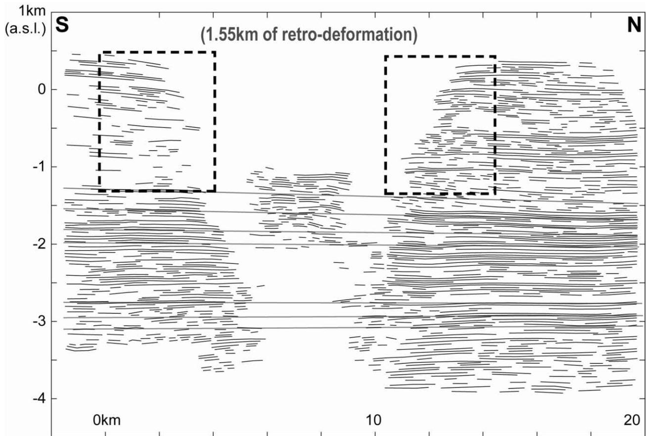
Figure 15: Anjihai seismic reflectors, retro-deformed using the parameters from figure 14 and the finite shortening deduced from figure 13. Shallow reflectors near fold core (dashed black boxes) have recorded only part of finite shortening, as evidenced by their retro-deformed dips.
