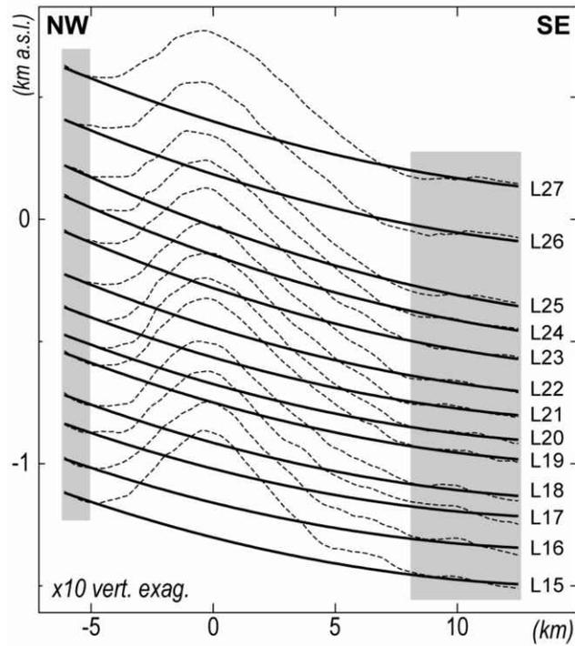
Figure 5: Regression of the original geometry of syntectonic seismic markers across Yakeng anticline. These second-order polynomial fits are constrained by data points away from the fold (gray boxes), and have different linear trends but a common quadratic component, thus similar curvatures (see details in text).
