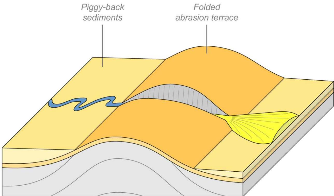
Figure 19: Surface expression of fold after relief emergence, corresponding to figure 18C. Sedimentation is perturbed by rapid accumulation of sediments upstream of fold, in piggy-back basin, and by secondary alluvial fans downstream of it.
