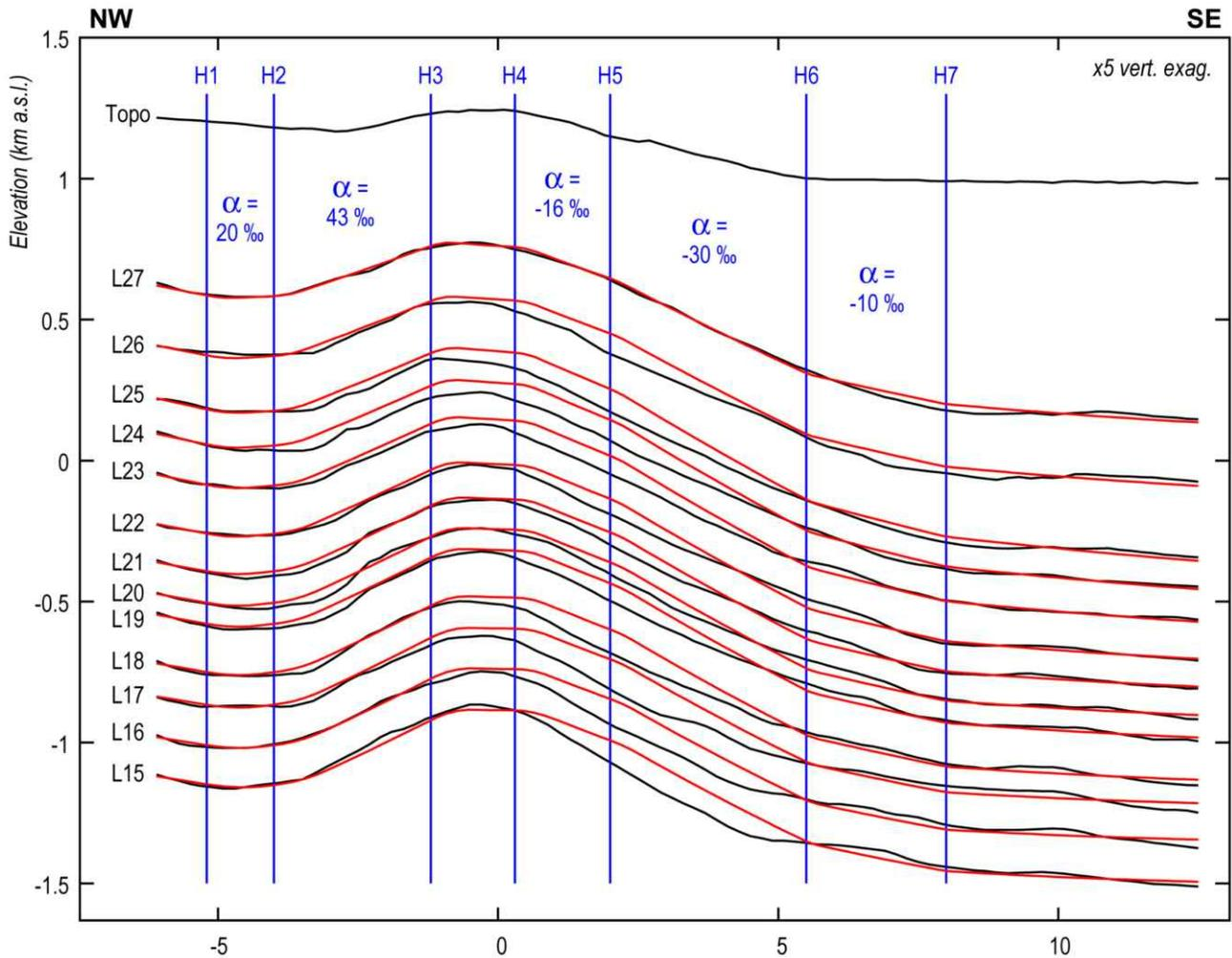
Figure 7: Parameters (in blue) of Yakeng deformation model. Black lines mark topography and observed seismic markers L15 to L27. Red lines mark the model-predicted geometry of markers, assuming the initial geometry shown in figure 5, and a constant shortening rate predicted by the linear regression of figure 6. We elected to primarily fit L27 rather than the more disturbed deeper markers (discussed in text).
