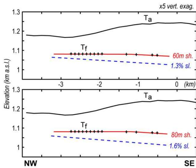
Figure 8: Models of deformed fluvial terrace Tf across Yakeng fold. Depending on the initial slope of the river terrace (1.3 to 1.6%, dashed blue, discussed in text), the amount of shortening necessary to deform it into its present-day geometry (black crosshairs) varies from  $60\pm 5$  m to  $80\pm 5$  m. Red lines plot the predicted Tf geometry.
