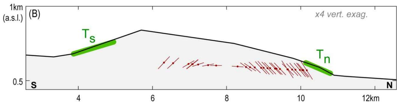
Figure 11: Geomorphic markers recording folding at Anjihai. (A) E-looking field photograph of loess-covered abrasion terrace  $T_n$ , unconformably overlying older alluvial gravel conglomerates exposed by fluvial incision. (B) Sketch of available surface records of folding. Black line follows topographic cross-section. Green segments mark positions of well-preserved terraces  $T_n$  and  $T_s$ . Red lines plot projected dips of surface structural measurements.
