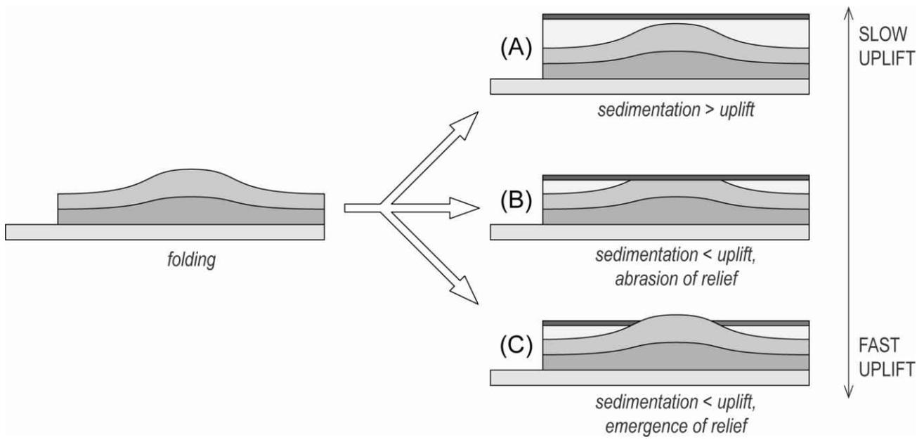
Figure 18: Summary of fold growth accounting for interactions between uplift, sedimentation and erosion (see discussion in text).
