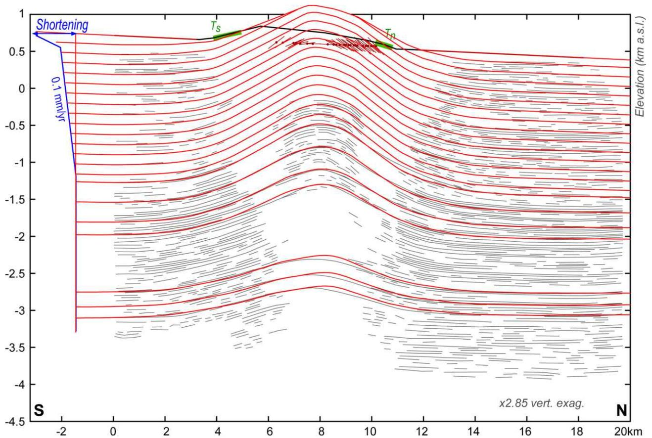
Figure 17: Predicted structure of Anjihai fold assuming a two-phase shortening history. This model fits the observed topography and structural dips, but fails to model  $T_n$  and  $T_s$  as a single, coeval surface.
