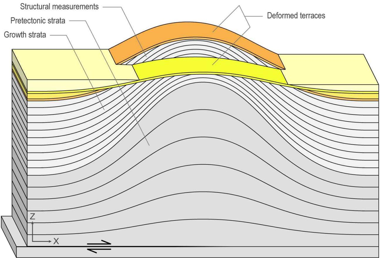
Figure 1: Synthetic sketch of the structural and geomorphic record of deformation, in the case of fold formed at the tip of a detachment fault.
