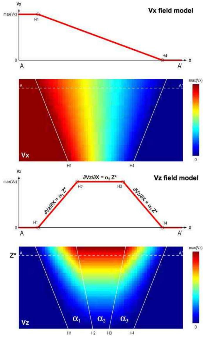
Figure A1: Simplified plot of Vx and Vz dependence on (X,Z) used in our folding models, modified from Bernard *et al.* [2006].
