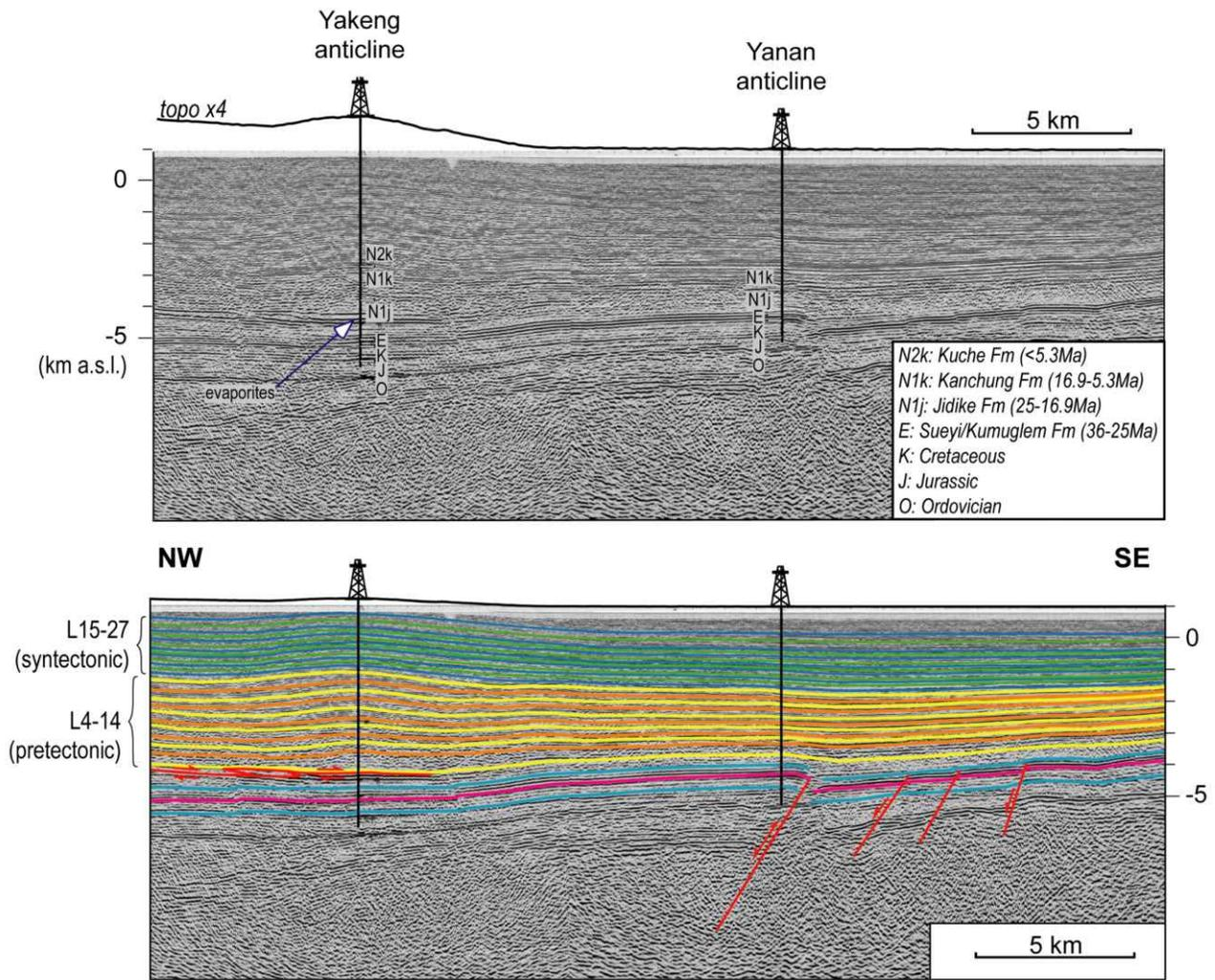
Figure 4: Seismic data and interpretation of Yakeng fold, from *Hubert-Ferrari et al.* [2005].
