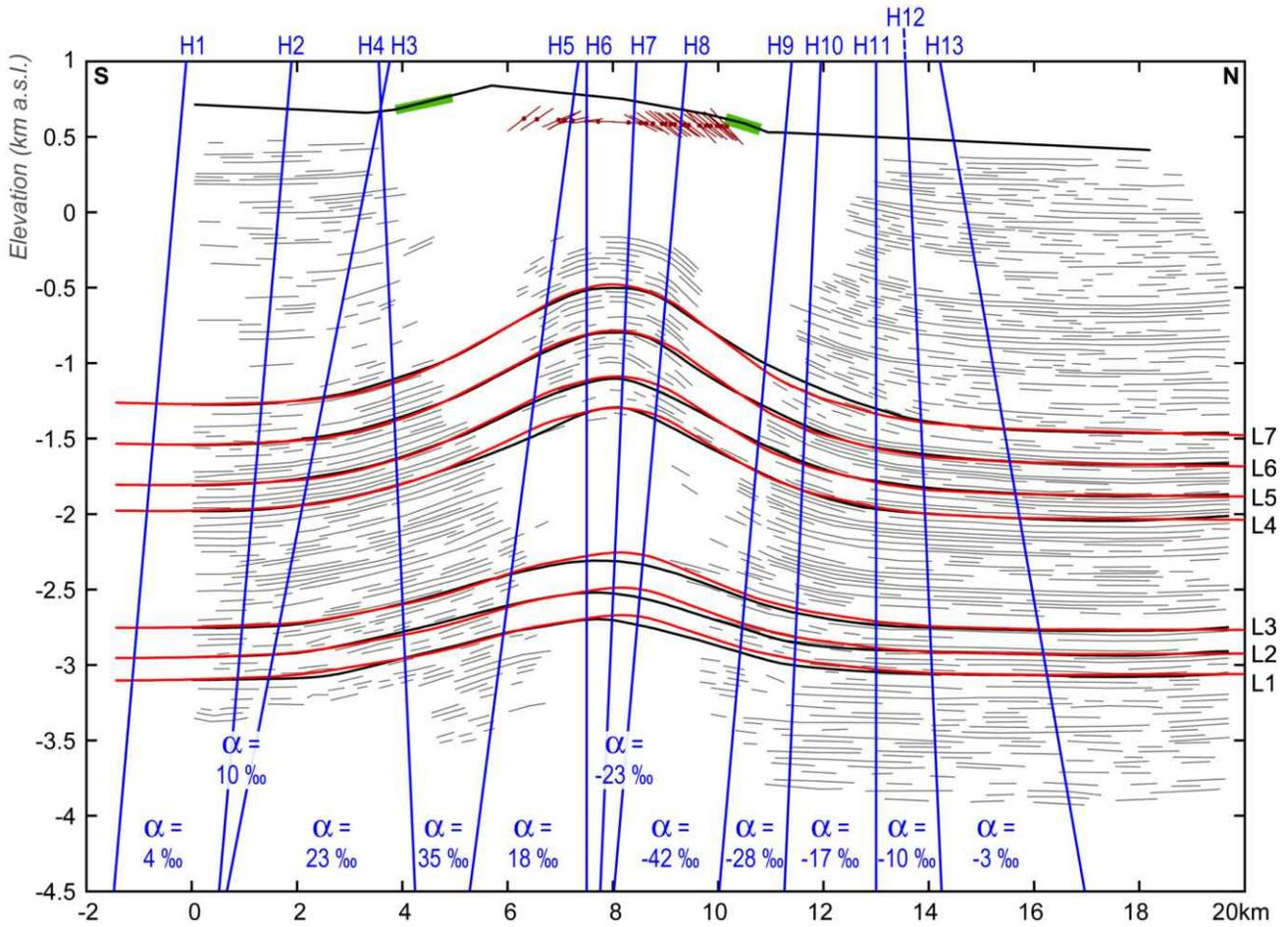
Figure 14: Parameters (in blue) of Anjihai deformation model. Black lines mark topography and observed continuous seismic reflectors L1 to L7. Red lines mark the model-predicted geometry of reflectors, using the finite shortening measured in figure 13.
