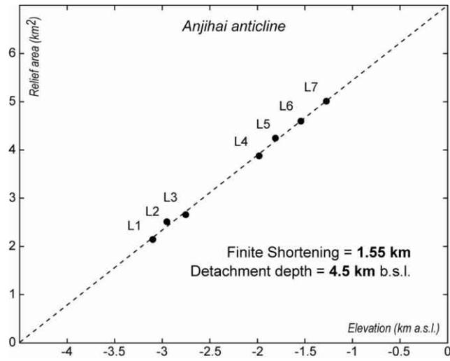
Figure 13: Plot of excess area versus stratigraphic depth for Anjihai fold. Linear fit corresponds to 1.55 km of finite shortening.
