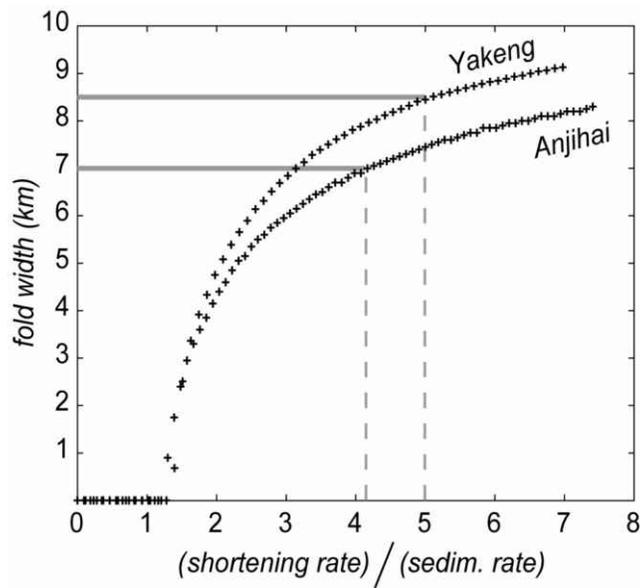
Figure 20: Predicted fold width at the initiation of relief emergence, as a function of the ratio of shortening and sedimentation rates. The observed fold widths correspond to ratios of 5.0 (Yakeng) and 4.15 (Anjihai). Combined with the relevant magnetostratigraphic sedimentation rates, these ratios imply modern shortening rates of 2.15 and 1.12 mm/yr, respectively.
