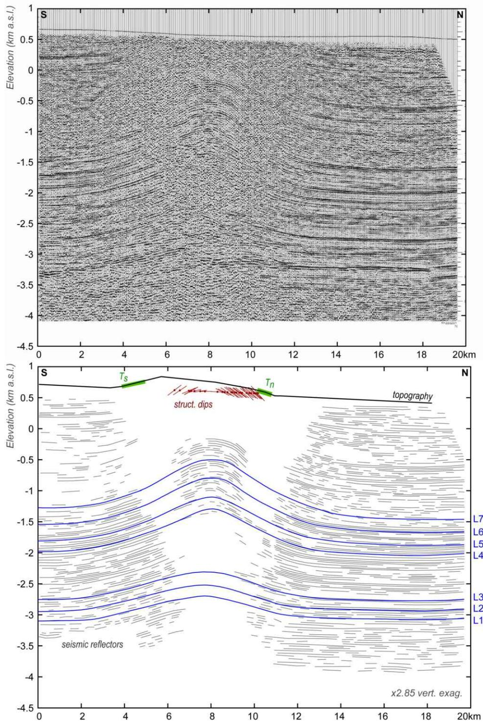
Figure 12: Seismic profile across Anjihai [Dengfa et al., 2005] and our line-drawing interpretation (grey segments). Seven continuous reflectors (blue lines L1 to L7) can be mapped across the fold.
