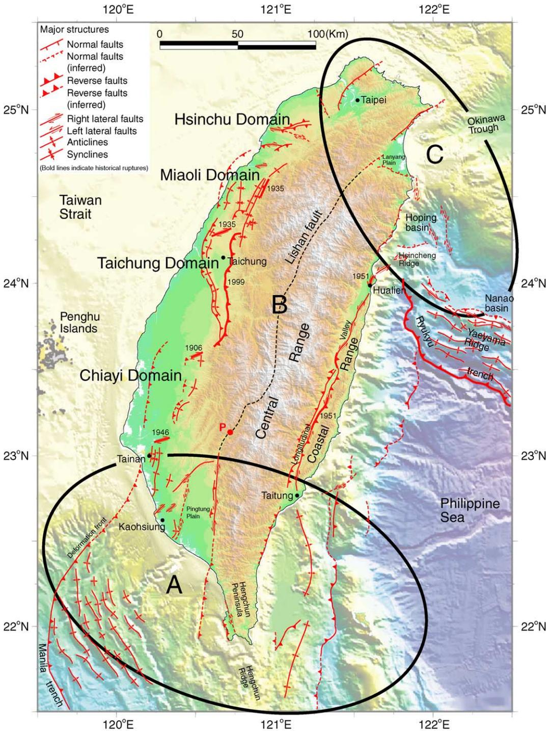
on the northwest by an active normal fault [28] that extends offshore as a minor fault on the continental shelf. This is consistent with GPS measurements, which show that the Taipei Basin is extending at low rates. Slip on this normal fault may have resulted in creation of a marine incursion into the basin in 1694 [29].
