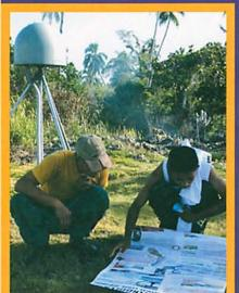
GPS stations, like this one on Tello (left), capture data from satellites. Scientists use the data to measure how much islands are sinking between earthquakes. Even without GPS, islanders knew the water level was changing. On Siberut Island (below), 29-year-old Tulik shows Kerry Sieh a well that gave freshwater when he was young. As the island sank, the well was flooded with seawater.
