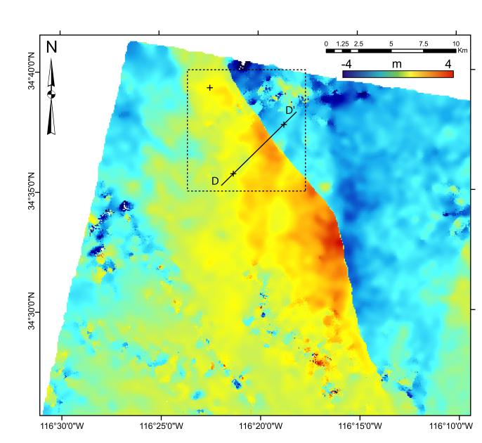
North/South component of the denoised SPOT correlation map. The GCPs are located away from the fault to assume a null ground displacement. Images are orthorectified on a 10 m resolution grid and correlated using a 32 × 32 pixels window with a 8 pixels step. The dotted square represents the air photo footprint, and black cross indicates the location of the air photo GCPs.
