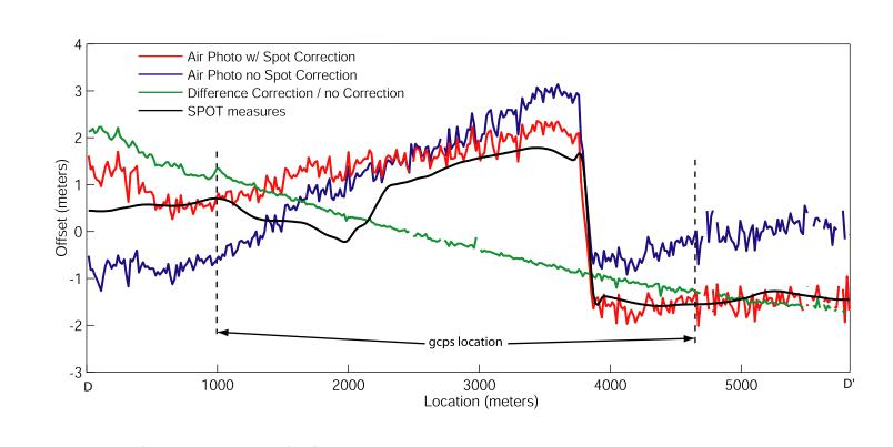
Profile DD'. GCPs correction brings a 2nd order polynomial correction in each NS and EW directions. High frequency signal (displacement at the fault) is not affected however.
