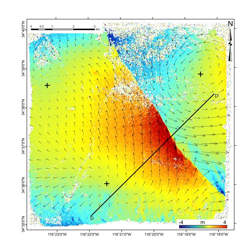
NS component of the correlation map. Three GCPs, located by the black crosses, are optimized to co-register the images without accounting for seismic ground displacement at their ground location. Arrows represent the ground displacement field accounting for both NS and EW components. Long wavelength distortions are introduced to satisfy the images co-registration.
