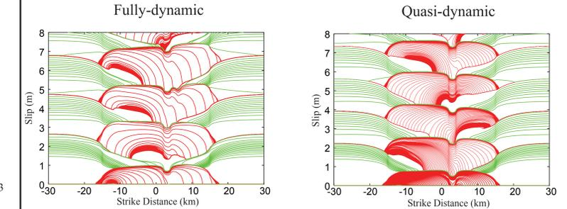
Fig 3: Accumulation of slip vs. strike, along the line  $z = -8$  km that passes through the center of the heterogeneity. The red lines are plotted every 1 second when the maximum slip rate exceeds 1 mm/s. The green lines are plotted every 5 years.
