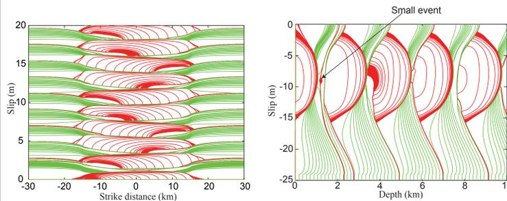
Fig 1: Accumulation of slip vs. strike, along the line  $z = -8$  km. The red lines are plotted every 1 second when the maximum slip rate exceeds 1 mm/s. The green lines are plotted every 5 years.
