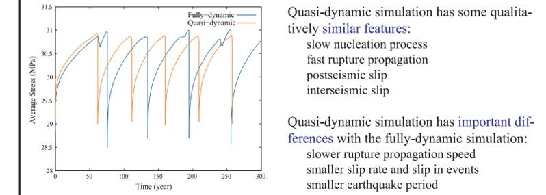
Fig 4: Comparison of average stress drop between fully-dynamic and quasi-dynamic models.
