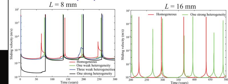
Fig 5: Sliding velocity evolution for several simulated cases with different heterogeneities on the fault. Every vertical line represents an event, and the time intervals between vertical lines are earthquake periods  $T$ . For  $L = 16$  mm,  $T$  is different for different cases. For  $L = 8$  mm,  $T$  is almost the same.
