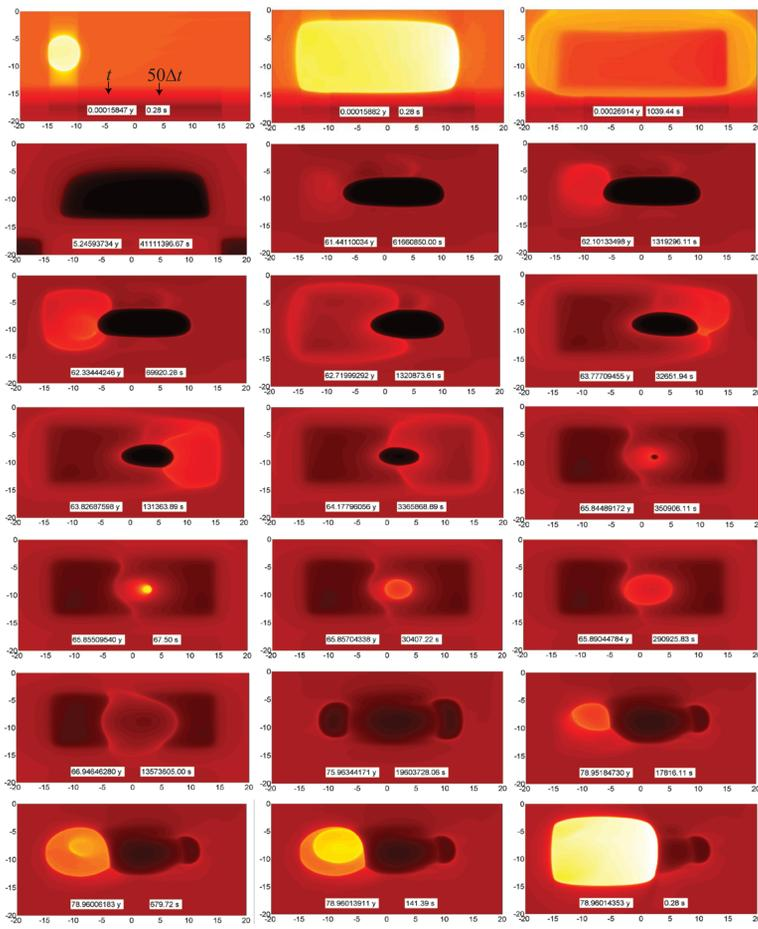
The color scheme depicts the slip rate in m/s on a logarithmic scale. Each snapshot has two time markers. The first one is simulated time  $t$  in years. The second one is the current time step  $\Delta t$  multiplied by 50.
